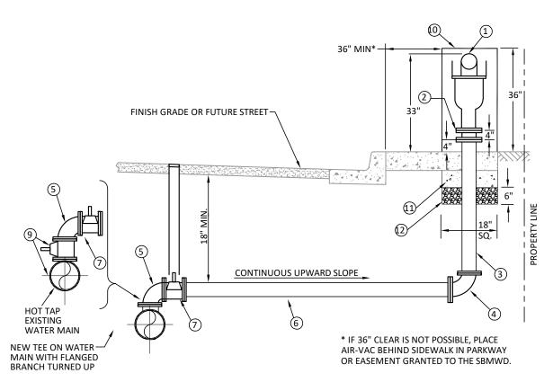
NOTE: PROVIDE ADEQUATE DRAINAGE FOR AIR VAC. IF ADEQUATE SURFACE DRAINAGE IS NOT PRACTICAL, USE A 2 CUBIC FOOT GRAVEL FILLED SEEPAGE PIT TO AVOID POSSIBLE DAMAGE CAUSED BY SURFACE WATER RUN OFF.
